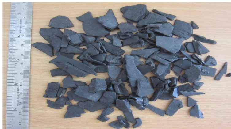
Fig. 6: Formation of e-waste plastic aggregate (Senthil Kumar & Baskar, 2015b).
