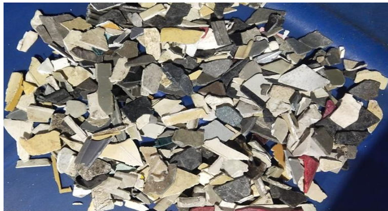
Fig. 5: Shredded e-waste plastic strip.
