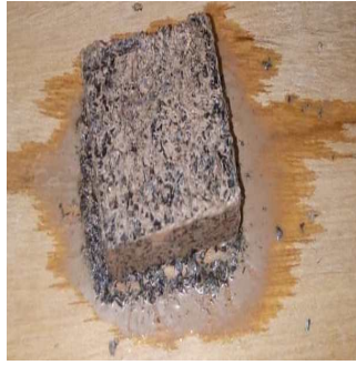
Fig. 10: Material loss during compaction of Bcp4 at m_{\text{water}} = 30\text{ g}
