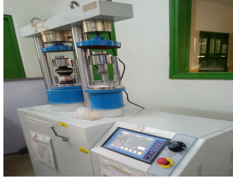
Fig. 3: Compressive strength tests with the UTEST (UTCM-6431, Ankara, Turkey) device
