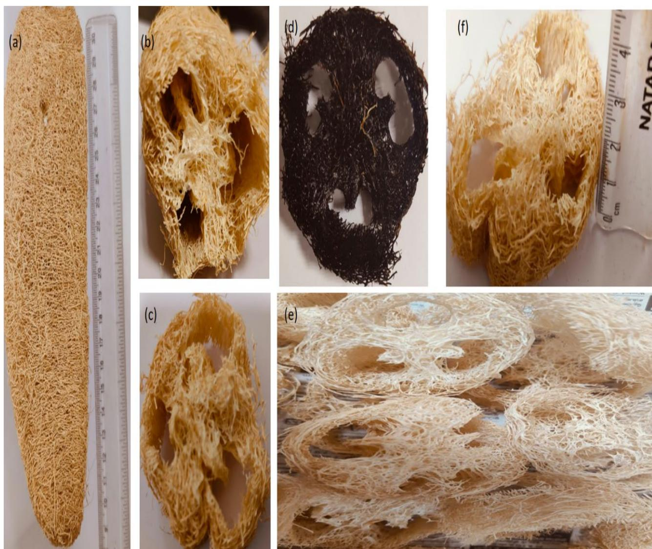
**Fig. 2: (a) LS (b) cross section of LS (c) cut piece of LS (d) alkaline, acid treated LS (e) KMnO<sub>4</sub> treated LS (f) SSGP-pretreated LS.**
