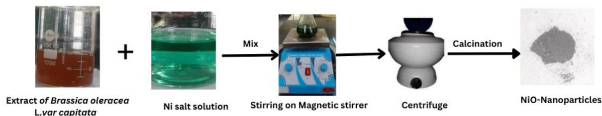
**Fig.1**-Schematic representation of preparation process of NiO-NPs
