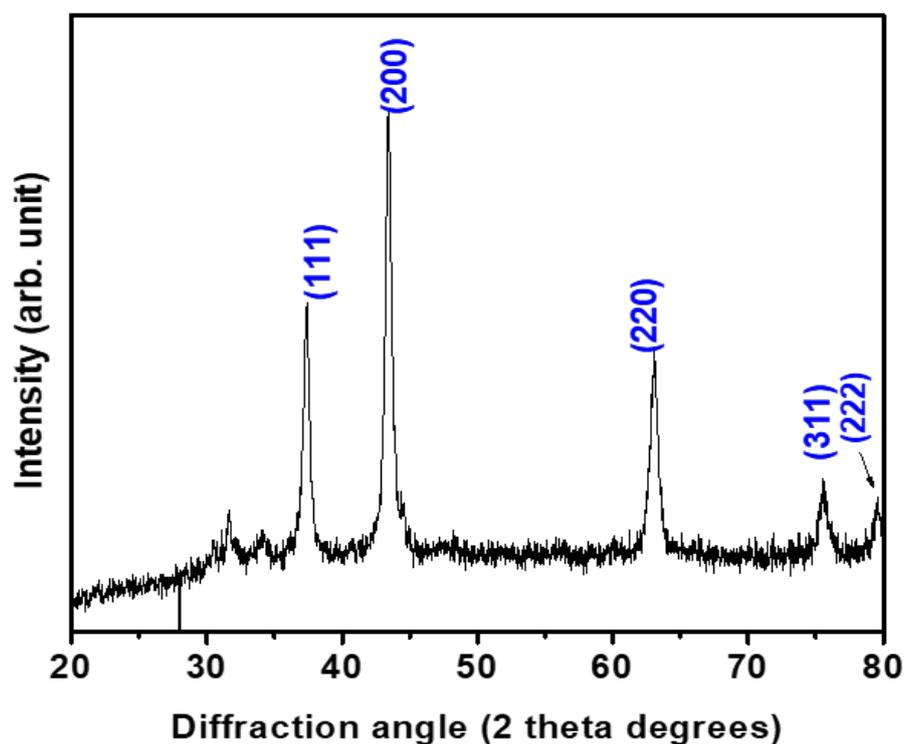
Fig.2- XRD pattern of green synthesized NiO-NPs
