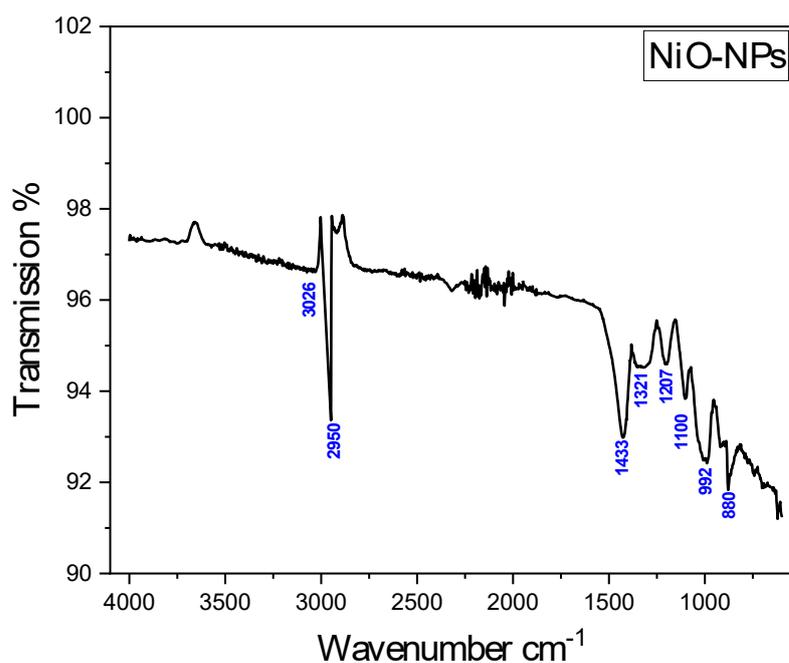
**Fig.4-**FT-IR Spectrum of Ni-NPs from *Brassica oleracea L. var. capitata*
