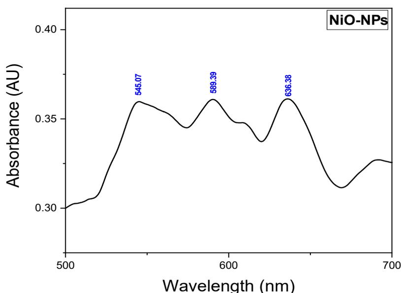
**Fig.3-** UV-visible Absorption Spectra of NiO-NPs
