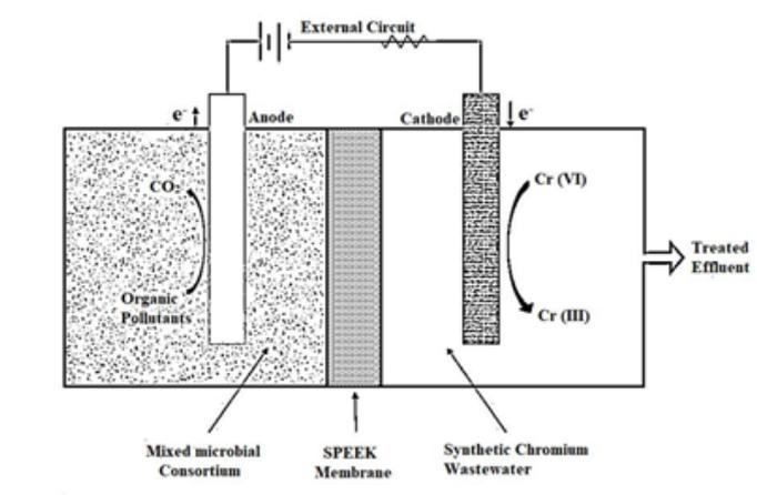
Fig.1: Microbial Fuel Cell
