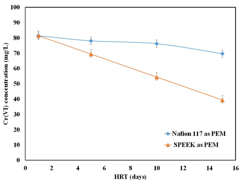
Fig 10. Biochemical reduction of Cr (VI) in both the reactors for HRT of 15 days at pH 2
