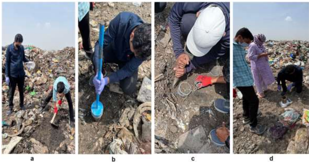
Fig. 3: Arranging the multi-step field process from left to right (a to d) a) Surface area cleaned and levelled, b) Core cutter driven into the soil using a dolly and rammer, c) Core cutter excavated and removed with surrounding soil, d) Core cutter with soil sample weighed.
