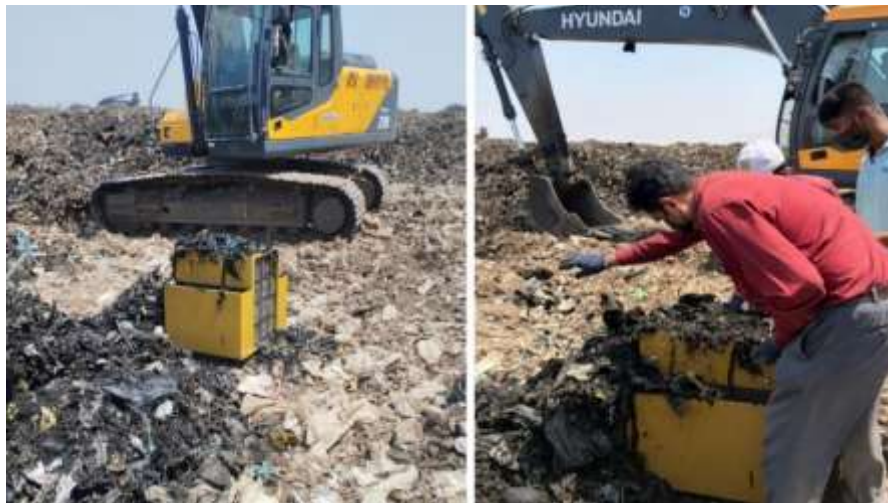
Fig. 2: Field-scale loading of the MSW sample into the designed permeameter.
