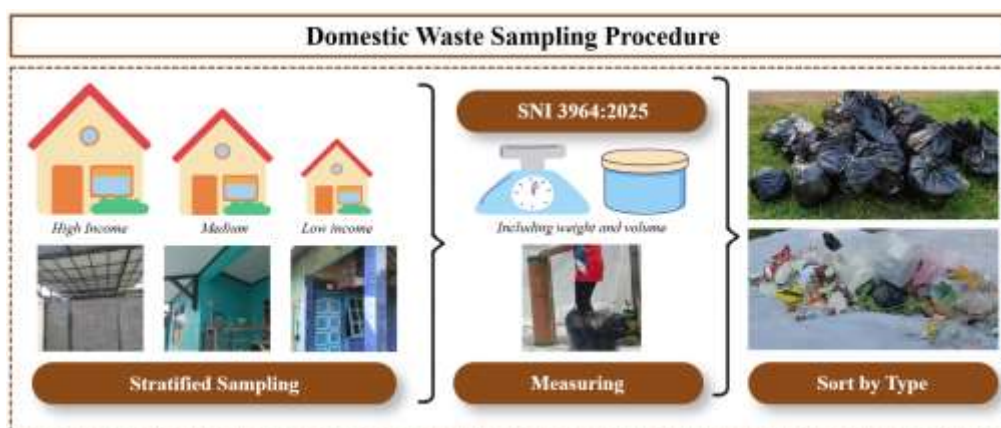
Fig 5: Domestic waste sampling procedure
