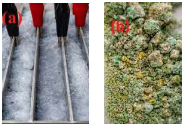
Fig. 10. (a) Floating flocs (b) Dried flocs formed during the electrocoagulation process.
