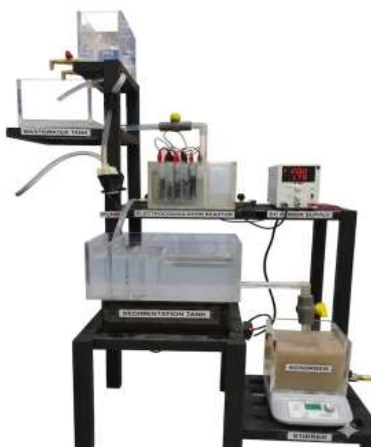
Fig. 1: Experimental setup of the integrated electrocoagulation–adsorption system.
