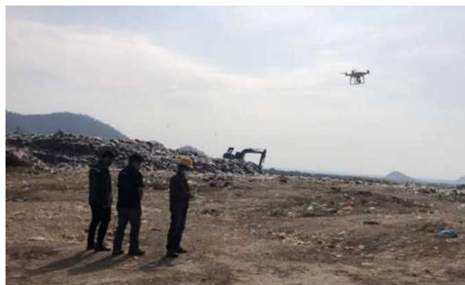
Fig. 3: Survey of the entire landfill site using a UAV (Unmanned Aerial Vehicle) in Kaeng Sian, Kanchanaburi.
