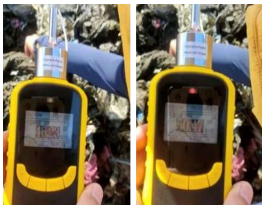
Fig. 4: SKY 2000-CH 4 ; Portable CH 4 methane gas analyzer with ATEX, CE, and ISO 9001 certification
