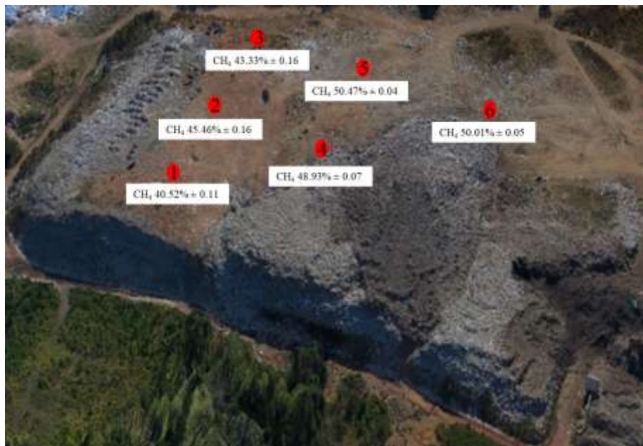
Fig. 8 Concentration of CH 4 gas at each point of the landfill site
