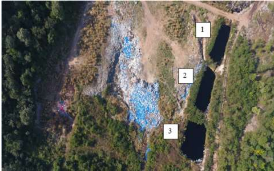
Fig. 9: Leachate ponds in the landfill area.
