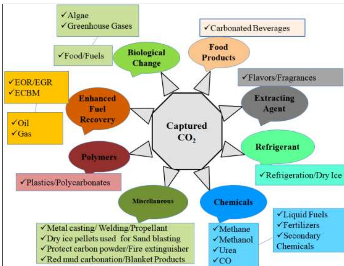
Figure 1. Illustration of various products that can be obtained from CO 2 -absorption technologies.
