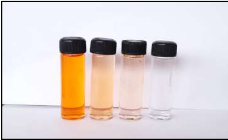
Fig. 8: Gradual colour changes from orange to colourless after the addition of iron
