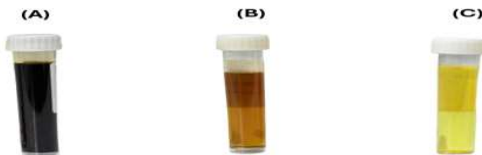
Figure 8: (A) spent oil, (B) Recovered base oil after bleaching, (C) Stock 60
