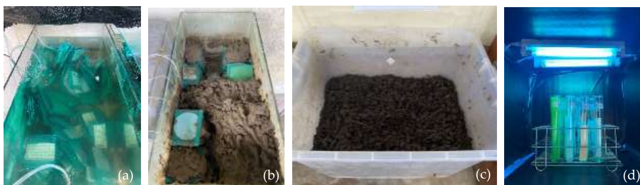
Fig.1: Exposure media (a) Freshwater (b) River Sediment (c) Compost (d) UV chamber
