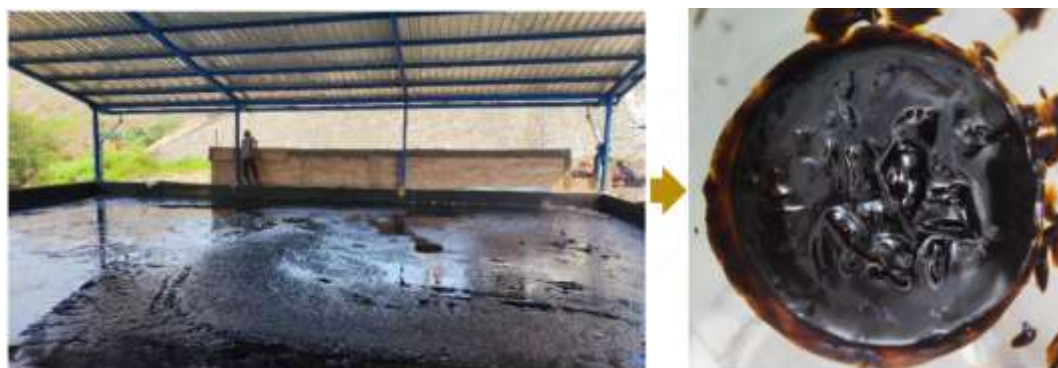
Fig. 1: Tar (by-product) from MSW gasification in Putri Cempo landfill, Indonesia.
