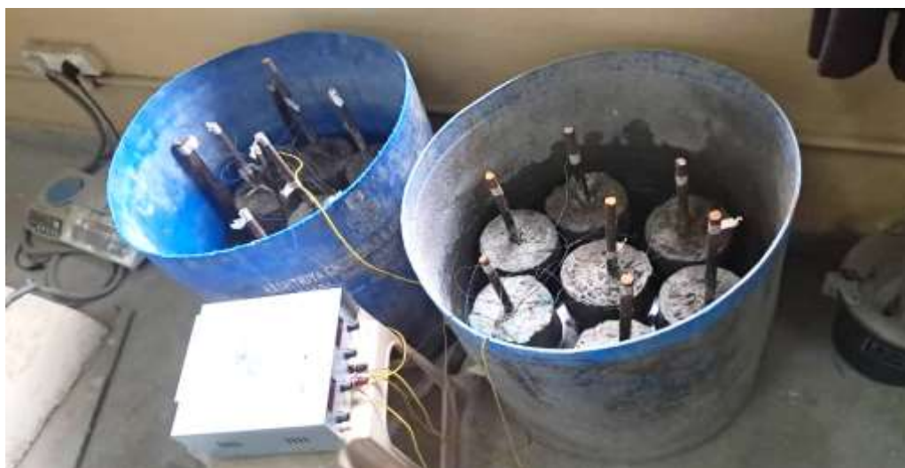
Fig. 5: Accelerated Corrosion Setup
